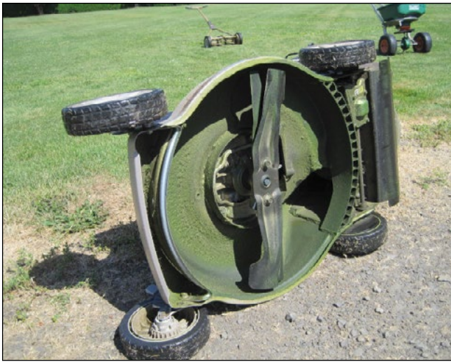
Figure 9. The double blade pattern of a mulching mower is designed to thoroughly mulch grass clippings.
