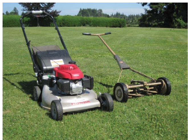
Figure 8: Rotary mowers (above left), while durable, typically cannot be set to a height below 1 inch. Push reel mowers (above right) typically cannot be set higher than 2 inches.
